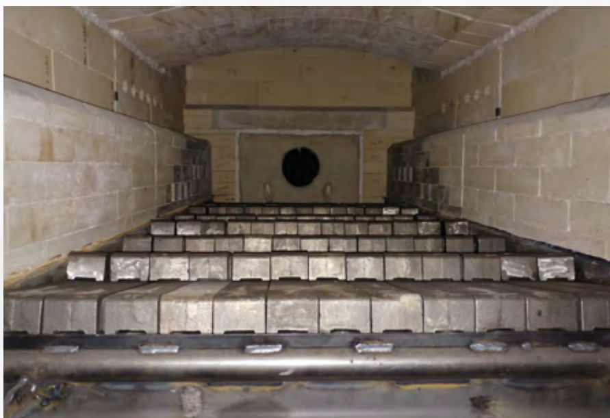
Combustion unit with hydraulically or electro-mechanically operated grate
